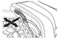
· The adjuster lever is spring loaded.
