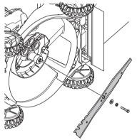
4 Use block of wood between blade and lawn mower housing and tighten the blade bolt, turning clockwise.
