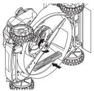
5 The bolt should be tightened with a torque of 35-40 ft. lbs. / 47-54 Nm.
