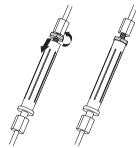
Make sure the drive control cable is not tensioned too tight. If the lawn mower starts to drive withtout the clutch lever is beeing operated, extend the wire.
