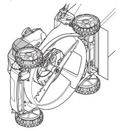
4 Use a wood block between blade and mower housing to prevent blade from turning when removing blade bolt.
