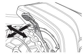
• The adjuster lever is spring loaded.
