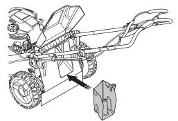
3 Allow the back shield to close and ensure the back shield is firmly shut against the mulch plug.
