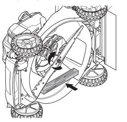
5 The bolt should be tightened with a torque of 35-40 ft. Ibs. / 47-54 Nm.
