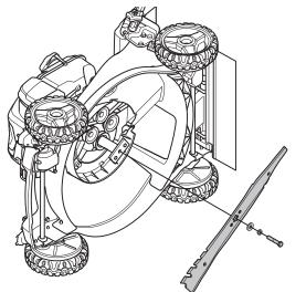
4 Use block of wood between blade and lawn mower housing and tighten the blade bolt, turning clockwise.
