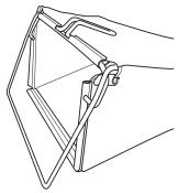
2 Secure the grass bag to the frame by using the quick-action clips.
