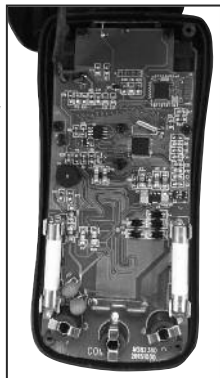
Where to find the DMM's cylindrical white ceramic fuses
