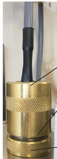
2) Quartz Sleeve inserted into UV Chamber Quartz Sleeve Black O-Ring Locking Nut
