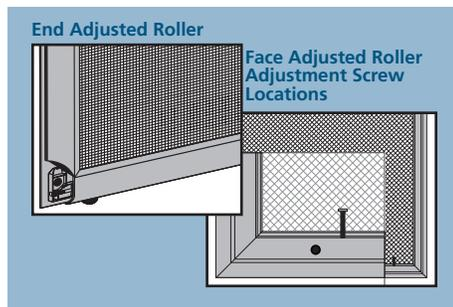
1. Turn all four adjustment screws to retract rollers into the screen.
