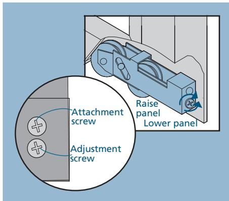
3. Lift the panel to take the weight off of the roller and turn the adjustment screw with a #2 Phillips head screwdriver (do not use a power driver). Clockwise rotations raise the panel, and counterclockwise rotations lower the panel.
