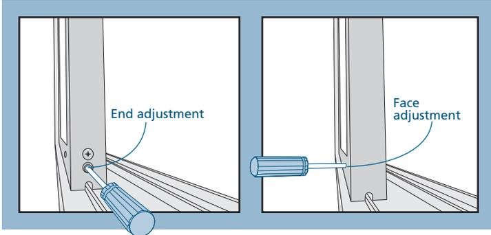
1. Builders doors have an adjustment screw on each lower end of the operating panel(s). Premium doors (and some older Builders doors) have access holes on the face of each lower end of the operating panel(s). Remove small vinyl plugs from each hole (if present).
