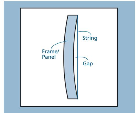
3. Look for gap between string and frame or panel. If gap measures more than 1/16" at any point, the panel is bowed.
