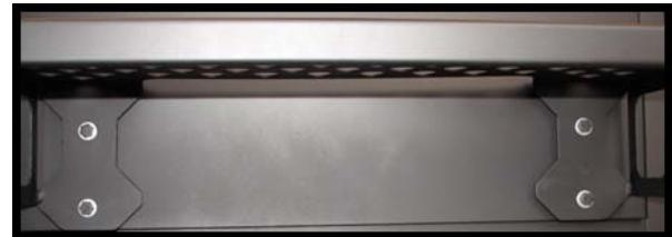
The shorter side shelf attaches to the four holes in the side of the grill. While holding up the shelf, insert and tighten the four washers and 1" long bolts, using a  $\frac{1}{2}$ " socket. (In case of the need to replace this part, use the reverse of this procedure.)
