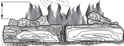
Figure 32 - Correct Burner Flame Pattern
