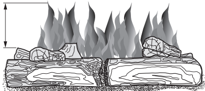
Figure 33 - Incorrect Burner Flame Pattern
