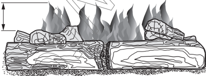
Figure 32 - Correct Burner Flame Pattern
