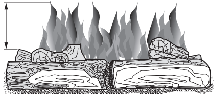
Figure 33 - Incorrect Burner Flame Pattern
