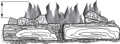
Figure 20 - Correct Burner Flame Pattern
