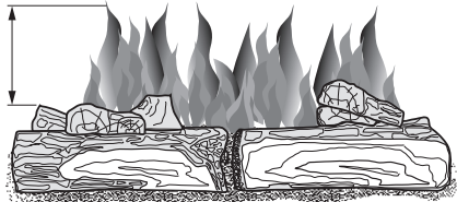
Figure 21 - Incorrect Burner Flame Pattern
