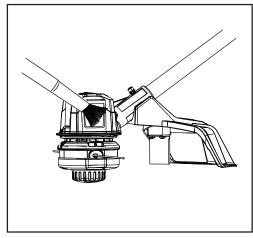
3. Clean line cutter blades by using a wire brush and spraying with an appropriate degreaser.
