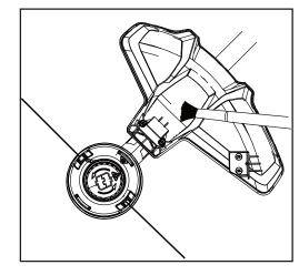
2. Clean dirt and debris off of motor cover and connection joints.
