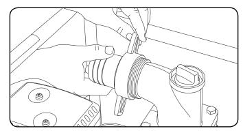
Slide the flexible, outlet hose over connector and secure with the hose clamp.
