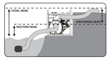
The pumping height, also known as the total head, is the distance from the water level to the point of discharge. As this distance increases, pump output decreases. The discharge capacity is greater than the suction capacity. Therefore, it is important that the suction head is less than the discharge head.
