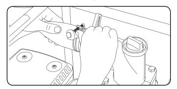
3. Attach the strainer to the intake hose and secure with the hose clamp.
