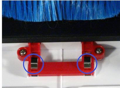
If bObi's dustbin is not fully engaged, her motor may not make proper contact with the battery's electrodes. If bObi does not restart her normal work after reinstalling her bin, or if she shows error 5 and her vacuum motor is not turning on, remove her dustbin, check that the connecting prongs on bObi are not stuck and can spring freely, then replace the dustbin securely.
