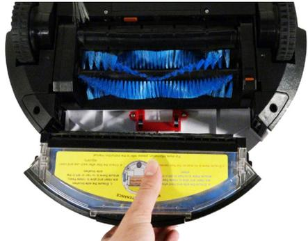
Hold the dustbin with both hands and press down the two colored clips on the sides of the dustbin to release its plastic door. For a quick clean, use the cleaning brush to remove the remaining dirt and dust from the dustbin.
