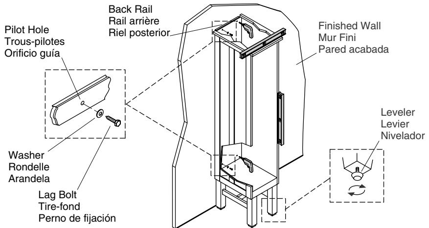
**WARNING:** Risk of property damage. Use care when moving the cabinet to avoid impacting, sliding, or side-loading the legs.
