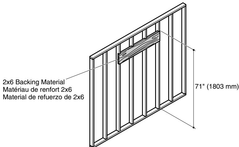
**NOTICE:** To properly secure the tall storage case, the top of the required 2x6 backing material must be 71" (1803 mm) from the finished floor.
