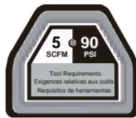
**IMPORTANT:** To operate correctly, this tool requires airflow of at least 5 Standard Cubic Feet per Minute (SCFM) at 90 Pounds per Square Inch (PSI) at the tool. The air hose length could affect how much air pressure the tool is actually receiving. You may need to adjust the air pressure higher on the air regulator to achieve the working pressure of 90 PSI.
