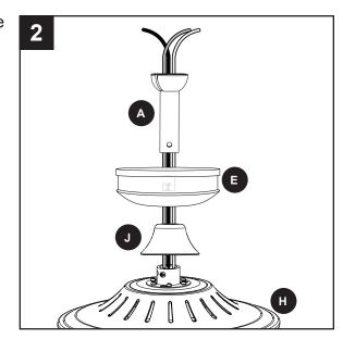
3. Slide the downrod (A) into the yoke of the motor assembly (H), align the holes, then re-install the downrod clip (C) and downrod pin (B). Secure with set the two screws (Q) and slide the yoke cover (J) down until it rests on top of the motor assembly (H).
