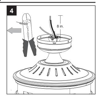
5. If you decided to cut back the lead wire in Step 4, strip 1/2 in. of insulation from the end of the white wire. Twist the stripped ends of each strand of wire within the insulation with pliers (not included). Repeat the step for black wire.
