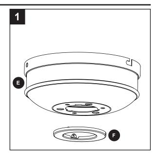
Remove three Phillips-head closemount screws (U) from the top of the motor assembly (H). Align the canopy (E) with the holes in the top of the motor assembly (H). Reinstall the closemount screws (U) to secure the canopy (E) to the top of the motor assembly (H).
