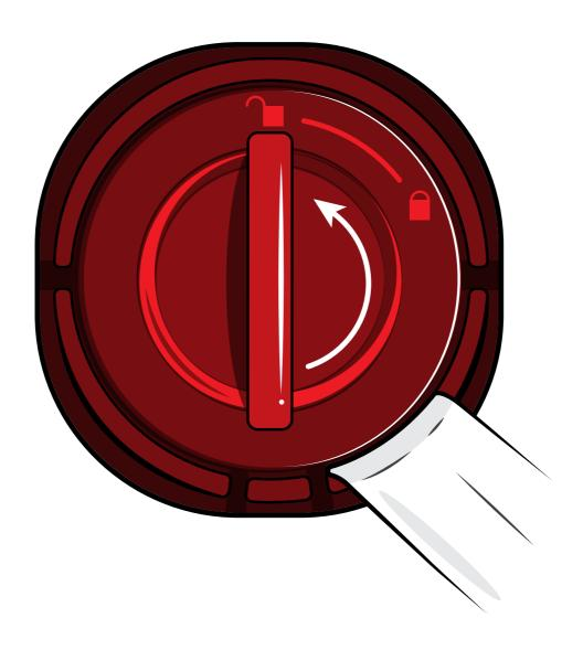
Remove the battery door from the underside of the iGrill Mini by twisting it anti-clockwise.
