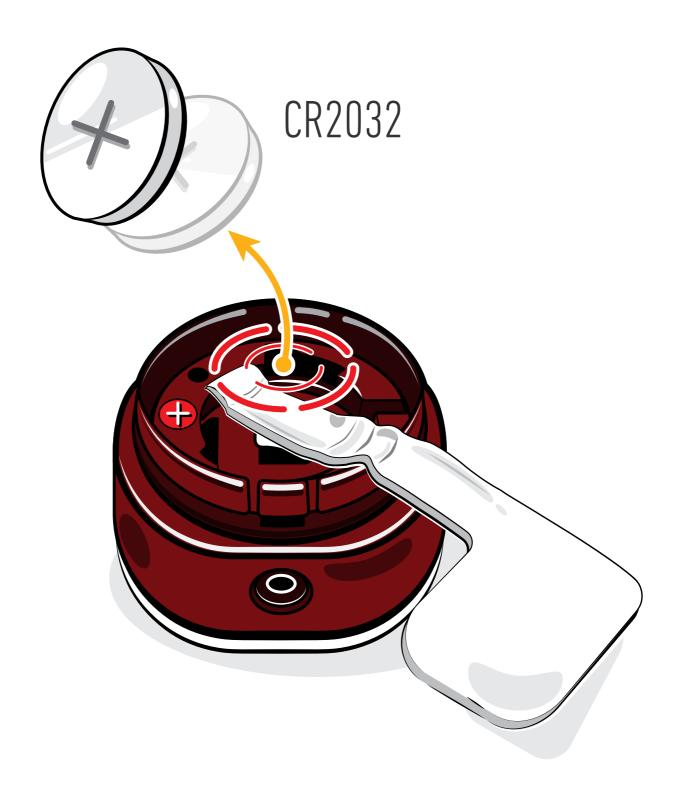
Pull the paper tab to remove the battery.
