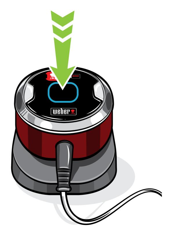
Quickly press and release the power button to turn on the iGrill Mini. The display will blink blue while it is waiting to pair.
