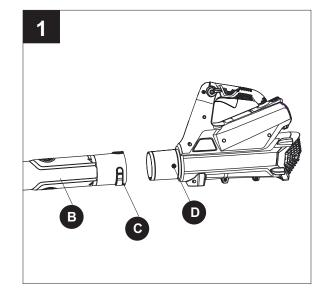
2. Turn the tube in the direction of the arrow until both of the tabs slide into locked position.
