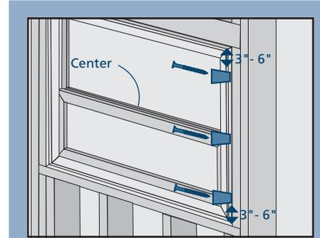
3. If installing a window using the stop in method, this installation assumes installation from the interior with exterior stops applied before window installation. All stops must overhang the window frame by a minimum of 1/8".
