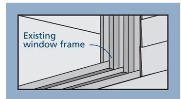
Flush fin windows must be installed onto a surface with at least a 3/8" wide exterior face. This face must be flush with or protrude past the exterior wall surface.
