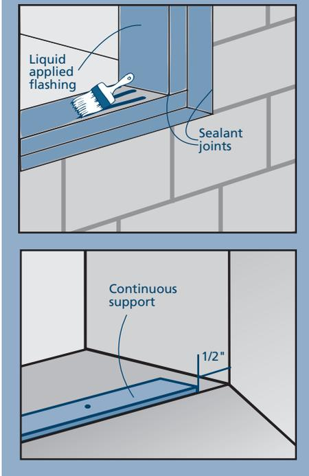
**Note!** Where the window will sit on the sill, shim to provide continuous support to the sill. This shimming must be 1/2" shorter than the width of the window frame, be 1/4" narrower than the depth of the window frame sill, should level the rough opening sill and be no more than 1/4" thick.
