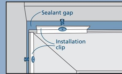
b. If installing a window with fasteners through the jambs, secure with a #8 screw until fully seated (without deforming vinyl).
