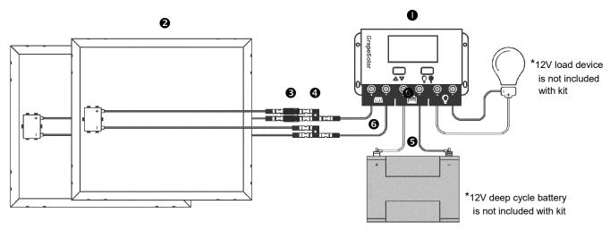
Remove the panel covering. In good sunlight, the charge controller's • "BAT %" should increase to 100%. When the controller is set to "LOAD ON," the system will provide power through the load control output or through the USB port.
