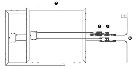
Connect the positive bare wire end **6** to the "+" PV input of the charge controller **0**.
