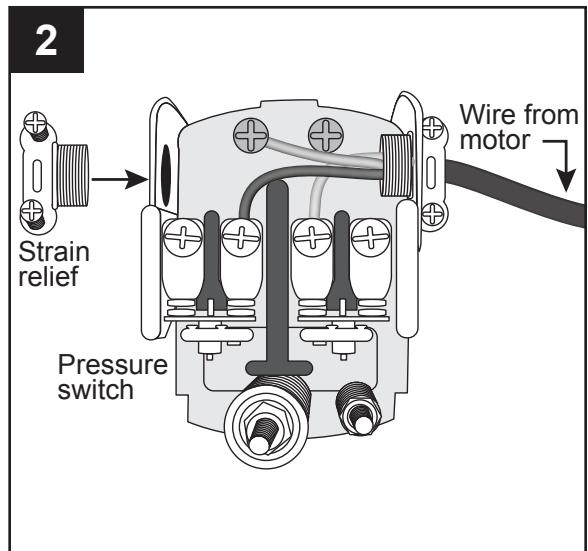
3. Thread the electrical wire (not included) from the power supply through the strain relief and tighten both screws on the strain relief. Do not crush wire.
