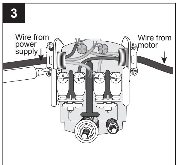
4. Connect the two wires from the power supply to the two outside terminals on the pressure switch.
