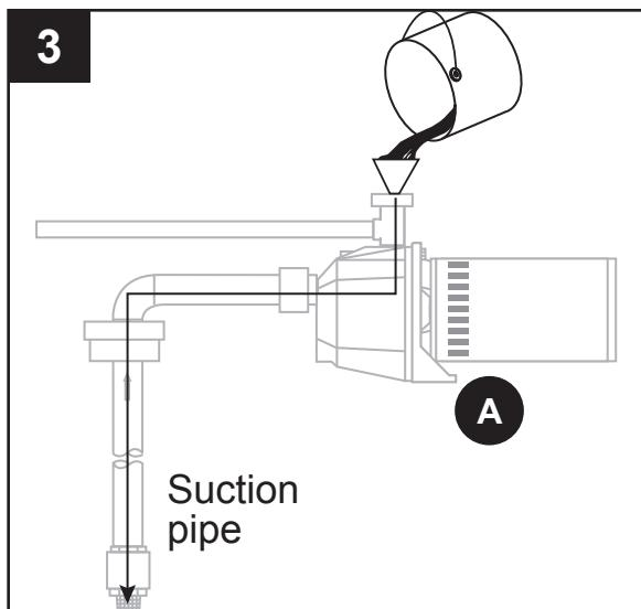
4. Check to be sure water in the cavity of pump (A) stays constant. If water level goes down, it could indicate a leak in the foot valve, check valve or suction pipe.
