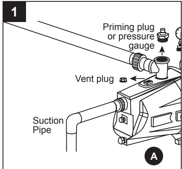
2. Slowly fill the discharge tee with water until water overflows the vent plug opening. Replace the vent plug loosely.
