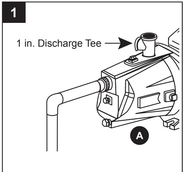
2. Install a 1 in. MPT x 1/4 in. FPT galvanized bushing and (optional) pressure gauge (both not included), or a pipe plug (not included). Do not tighten, as you will prime pump (A) later at this location.
