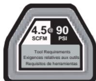
**IMPORTANT:** To operate correctly, this tool requires airflow that is at least 4.5 cubic feet per minute (SCFM) at 90 pounds per square inch (PSI). Check the specifications of your air compressor to be sure that it can support both the minimum SCFM and PSI required. The air hose length could affect how much air pressure the tool is actually receiving. You may need to adjust the air pressure higher on the air regulator to achieve the working pressure of 90 PSI.
