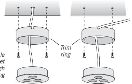
Feed power cable through cabinet surface or through notch in trim ring
