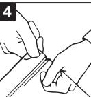
**4** Hold the two sides of the glass between your thumb and forefinger and bend slightly until it comes apart cleanly.
