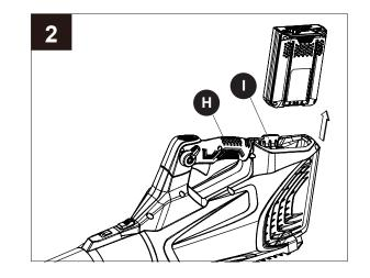
**Note:** The battery fits into the handle snugly in order to prevent accidental dislodging. It may require a strong pull to remove it.
