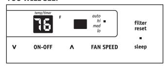
Note: In this mode the selected temperature will increase by 2 °F 30 minutes after the mode is selected. The temperature will then increase by another 2 °F after an additional 30 minutes. This new temperature will be maintained for 7 hours before it returns to the originally selected temperature. This ends the "Sleep" mode and the unit will continue to operate as originally programmed. The "Sleep" mode program can be cancelled at any time during operation by again pressing the "Sleep" button.
