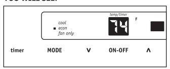
Note: In this mode, the fan will continue to run for 1 minute after the compressor shuts off. The fan then cycles on for 20 seconds at 10 minute intervals until the room temperature is above the set temperature, at which time the compressor turns back on.
