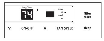
Note: Tap or hold either up (  $\Lambda$  ) or down ( V ) button until the desired temperature is seen on the display. This temperature will be automatically maintained anywhere between 60 °F (16 °C) and 90 °F (32 °C) . If you want the display to read the actual room temperature. See "To Operate on Fan Only" section on Page 7.
