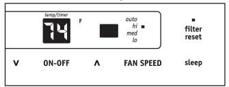
Note: This feature is a reminder to clean the Air Filter (See Care and Cleaning) for more efficient operation. The LED (light) will illuminate after 250 hours of operation. To reset after cleaning the filter, press the "Filter Reset" button and the light will go off.
