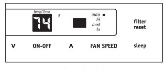
Note: Fan starts at High Speed and adjusts to a slower speeds the room temperature dictates. For example, if the room doesn't get too warm, it will stay at the slowest speed. If the room temperature rises quickly, such as a door being opened, it will automatically go to the highest speed. The fan speeds will re-adjust back to the slowest speed as the room returns to the original set temperature. Press either the fan slower or fan faster button to adjust the fan speed manually.
