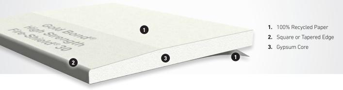
Use it for interior, 30-minute fire-rated and 1-hour fire-rated wall applications or non-rated ceiling applications. Gold Bond<sup>®</sup> High Strength Fire-Shield 30® has a fire-resistant, non-Type X gypsum core. This gypsum board is 30% lighter in weight than standard 5/8" (15.9 mm) Type X gypsum board.
