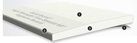
Use it for interior, fire-rated wall and ceiling applications. Gold Bond® High Strength Fire-Shield 60® features a Type X fire-resistant core for use in laboratory tested, fire-rated assemblies. This gypsum board is 20% lighter in weight than standard Type X gypsum board.
