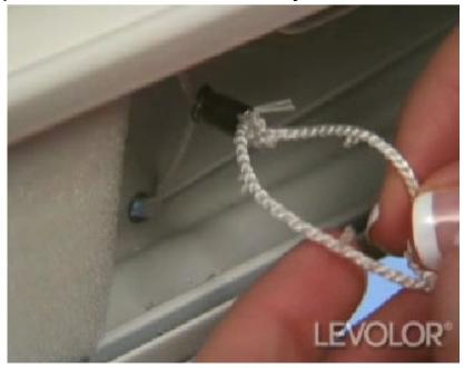
Step 12: Making sure all cords are tucked into the bottom rail, slide the bottom slat back into the bottomrail
