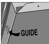
Figure 1 Face of wall can must extend 1/2" from face of stud to allow for sheetrock.
