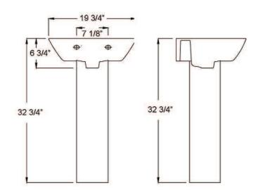
Dimensions of fixture are nominal and may vary within the range of tolerances established by ASME Standard A112.19.2-2008. Dimensions and specifications subject to change without notice.
