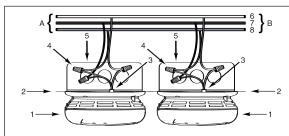
A. Unswitched 120VAC 60 Hz source B. To additional units; Maximum = 18 total (Maximum 12 Smoke Alarms)
