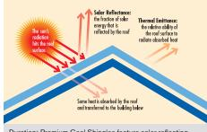
Duration\* Premium Cool Shingles feature solar reflecting granules that help keep roofs up to 10°F cooler for a more comfortable living space below.\*
