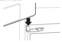
1 Lower the door onto the middle hinge pin.
