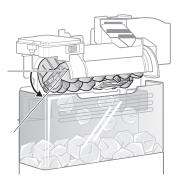
The ice-detecting sensors will sense when the ice is ready to be dumped into the ice bin.
