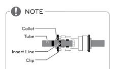
1) Gently press the Collet and insert the tube until only one line shows on the tube.
