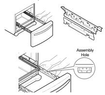
6 With the drawer pulled out to full extension, insert the lower basket (4) in the rail assembly.
