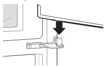
1 Lower the door onto the middle hinge pin. Make sure that the plastic sleeve is inserted into the bottom of the door.
