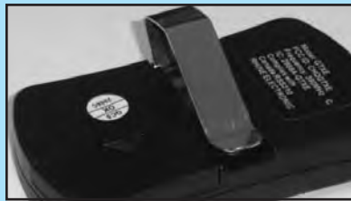
FIG. 8-3 Attach visor clip.
