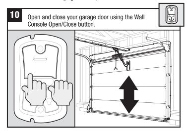
**NOTE:** Using these functions for the first time automatically sets the Force needed to open and close your garage door.
