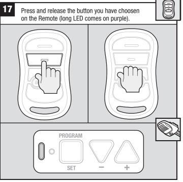
**NOTE:** Do NOT hold Remote too close to the Powerhead when programming Remote buttons.
