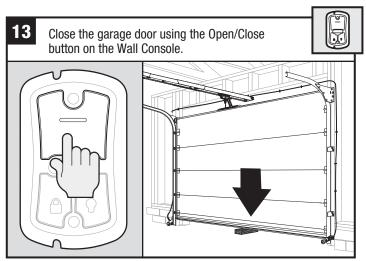
When the door contacts the board, it should stop and reverse direction within 2 seconds to the fully OPEN position.
