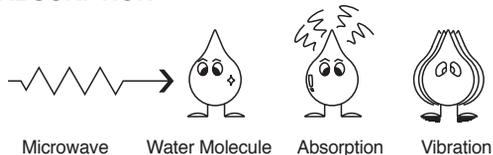
The microwaves cause the water molecules to vibrate which causes **FRICTION**, i.e. **HEAT**. This heat then cooks the food. Microwaves are also attracted to fat and sugar particles, and foods high in these will cook more quickly. Microwaves can only penetrate to a depth of 4-5cm and as heat spreads through the food by conduction, just as in a traditional oven, the food cooks from the outside inwards.
