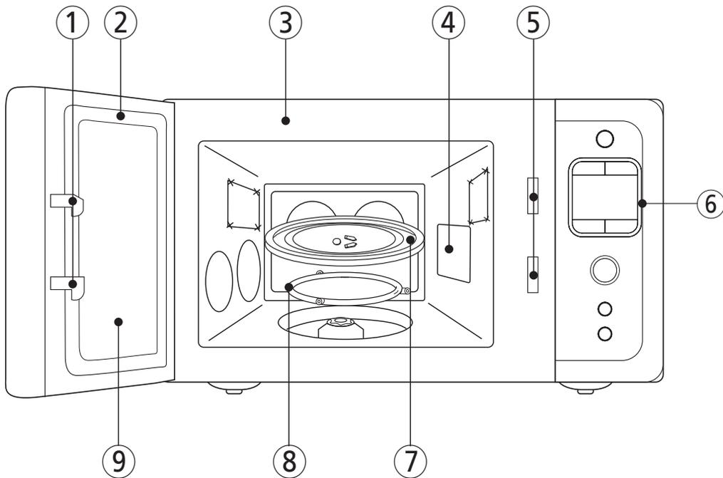
① **Door latch** - When the door is closed it will automatically shut off. If the door is opened while the oven is operating, the magnetron will automatically shut off.
