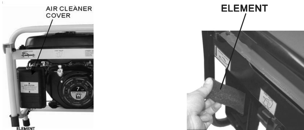
Figure 23- Removing the air cleaner casing.
