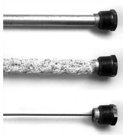
Figure 32 - Anode Rods from new (top) to partially depleted (middle) to fully depleted (bottom).
