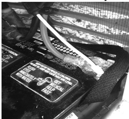
Figure 3.17 - Reconnect Battery Cables.
