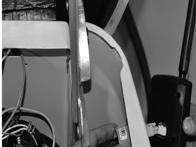
Figure 3.10 - Plug Harness into Mobile Link unit
