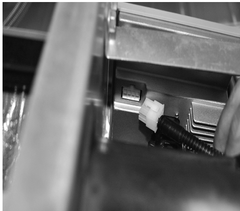
Figure 3.15 - Harness Installed to Controller.
