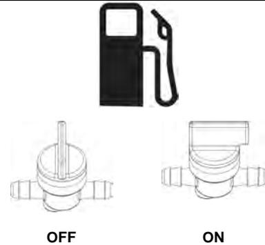
Add gas to fuel tank. Turn fuel valve to the ON position.
