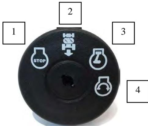
To start the machine set the throttle to fast and engage the choke. Turn the Ignition Key to position four until the engine fires. Disengage the choke after engine is running. **NOTE:** To mow in a generally rearward direction, turn the key to position two. To turn off the engine return the key to position one.
