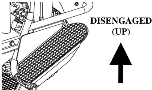
Before attempting to operate or work on the machine, be sure that the drive pedal located at the lower right side of the machine is fully disengaged in the UP position.
