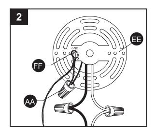
3. Supply wire connection guide: Make wire connections, securing with wire connectors (AA), following the reference chart listed below.
