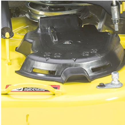
Spindle pockets on the 42A Mower
