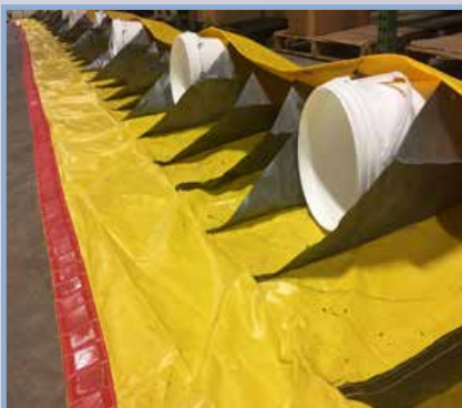
Place objects to raise Water-Gate to dry out, prior to storage
