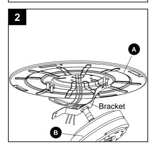
3. Connect the supply **GROUNDED/GREEN** wire to the **GREEN/GROUNDED** wires from the motor bracket using the wire connector (AA). Connect the fan motor **WHITE** wire to the supply **WHITE** wire using the wire connector (AA). Connect the fan motor **BLACK** and **BLUE** wires to the supply **BLACK** wire using the wire connector (AA).
