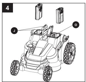
**WARNING:** Make sure the latch on top of the battery with battery release button snaps in place and the battery is fully seated and secure in the mower's battery port before beginning operation. Failure to securely seat the battery could cause the battery to fall out, resulting in serious personal injury.
