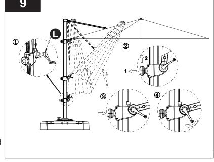
9. Insert crank (L) into the handle of the umbrella. Open the umbrella canopy by pulling up the button and lifting upward to raise the canopy. Release the button to set in the desired position.
