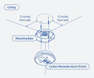
2. Fit the alarm inside the base by aligning it over the base, then turn the alarm in a clockwise direction until it clicks into place. The three LEDs will flash while the alarm powers up.
