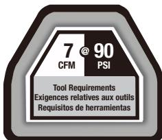
**IMPORTANT:** To operate correctly, this tool requires airflow that is at least 7 cubic feet per minute (CFM) at 90 pounds per square inch (PSI). Check the specifications of your air compressor to be sure that it can support both the minimum CFM and PSI required. An air hose may cause up to 15 PSI drop in pressure, so you may need to set the output higher to maintain the required pressure at the tool.
