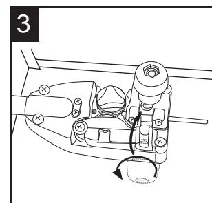
Once tension arm is up, open swing arm (H) so that welding wire can be fed through the wire feed assembly (F).
