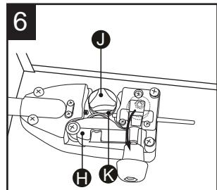
Feed welding wire through feed tube (I) and along the top groove of feed wheel (K).
