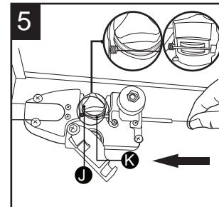
Before feeding the welding wire through the wire feed assembly, make sure to securely hold onto the end of the welding wire while keeping consistent pressure on the welding wire during the installation process. If consistent tension is not applied on the welding wire, the welding wire can spring backwards, causing a "bird's nest" in which the welding wire can bunch together, causing severe tangling resulting in wasted wire.
