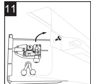
Once the welding wire is properly secured, loosen the thumb nut to remove the welding wire spool from the wire spool axle. Loosen the tension adjustment knob by turning it counterclockwise and raising up the tension adjustment knob.
