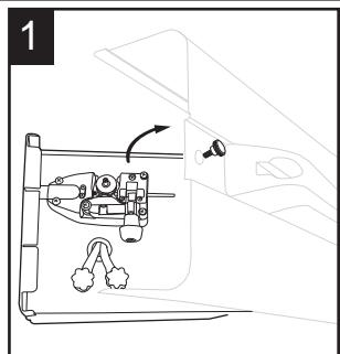
Unscrew the thumb nut (O) and remove top of spool knob and spring. Install a 2 lb. spool of welding wire (not included) on the wire spool axle (N). Secure the spool of welding wire to the wire spool axle (N) using the spring underneath and the knob on top. Tighten the thumb nut (O) by hand until only there is a slight resistance when turning the spool.
