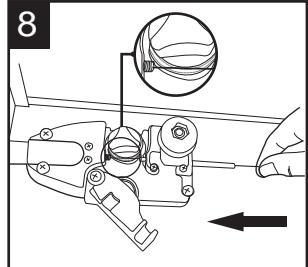
Once the wire has been fed into the wire feed inlet (L), close the swing arm (H) and then lower tension arm and slightly tighten adjustment knob (G).
