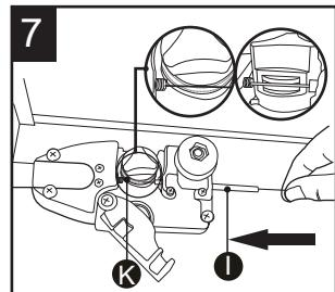
Continue to feed welding wire through and into the feed wire inlet (L).
