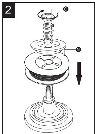
Loosen the tension adjustment knob by turning it counterclockwise then lift the tension adjustment arm up.
