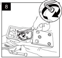
Install the spacer(part 56 shown on parts list of manual) by tighting 2 screws turning clockwise.(See Figure 9)
