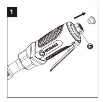
Mount a male plug (not included) by hand into the air inlet (E) (See Figure 2).
