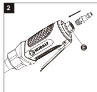
Place 2 - 3 drops of air tool oil (not included) into the male plug before each use (See Figure 3).
